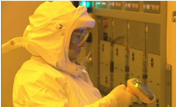
Inside an Intel fab, a technician works in a clean suit, or “bunny suit.” Image courtesy of Intel.
